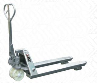
Hydraulic Pallet Trucks from 'JAY' are the most economical and cost effective solution for many transport application involving short distances. Its high capacity of two and half tons and easy manoeuvrability in small spaces makes hydraulic pallet truck the perfect warehouse equipment.
